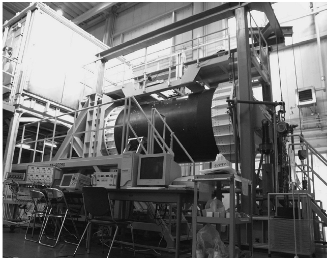
Figure 5. Set-up of Damage Detection and Suppression Demonstrator (Mitsubishi Heavy Industries, Ltd.).
